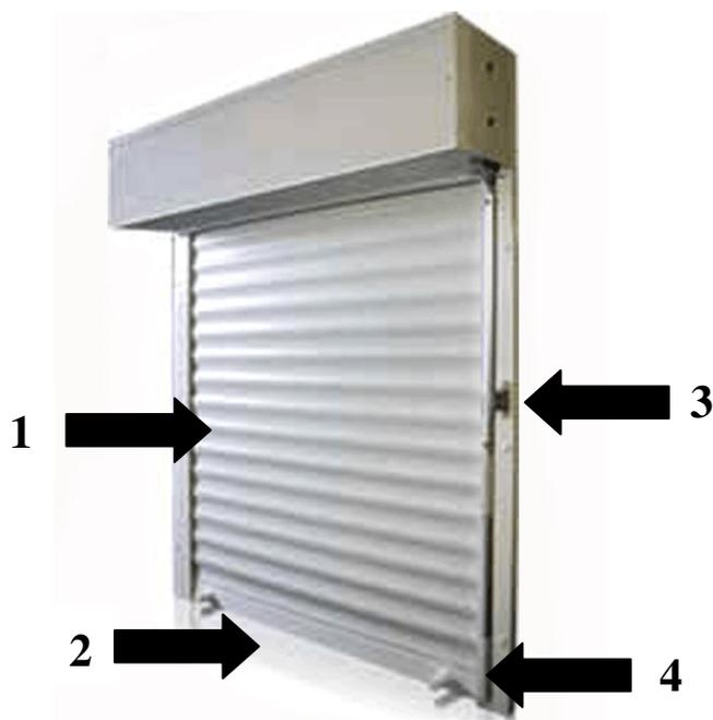
1. Check roll-up sections for damage. Holes larger than 1/4" must be repaired with metal. Roll-up sections with excessive damage should be replaced.
