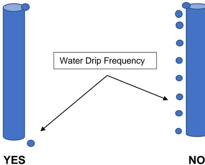
When compensating for Shut Off Valve leak, make a final adjustment of the bleed valve assembly to allow a drip of water coming out at a time from the reference tube (see diagram above). If the check valve is operating properly, the reading of the differential pressure gauge should be 1.0 psi or greater and recorded as the static pressure across the check valve.
