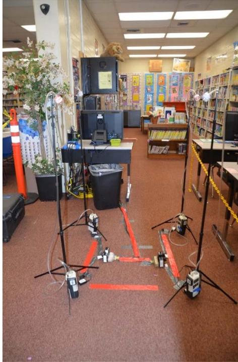
Photo 3 – Lincoln ES, Room 3 (Computer Room/Library), Air sampling and replicate air samples.
