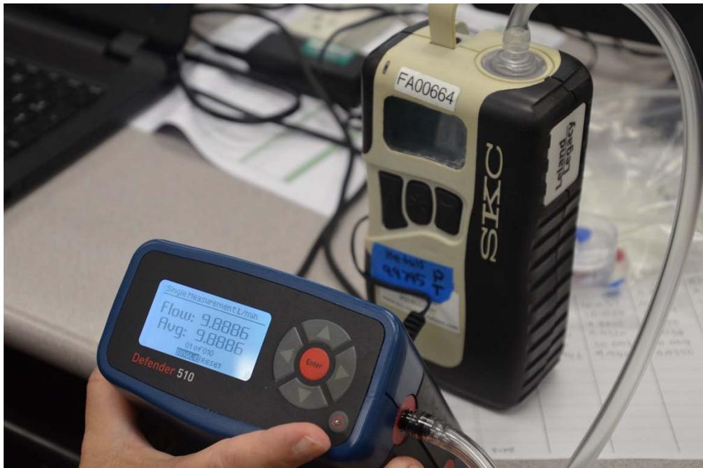
Photo 1 – Equipment calibration with a direct read primary standard traceable to NIST<sup>11</sup>
