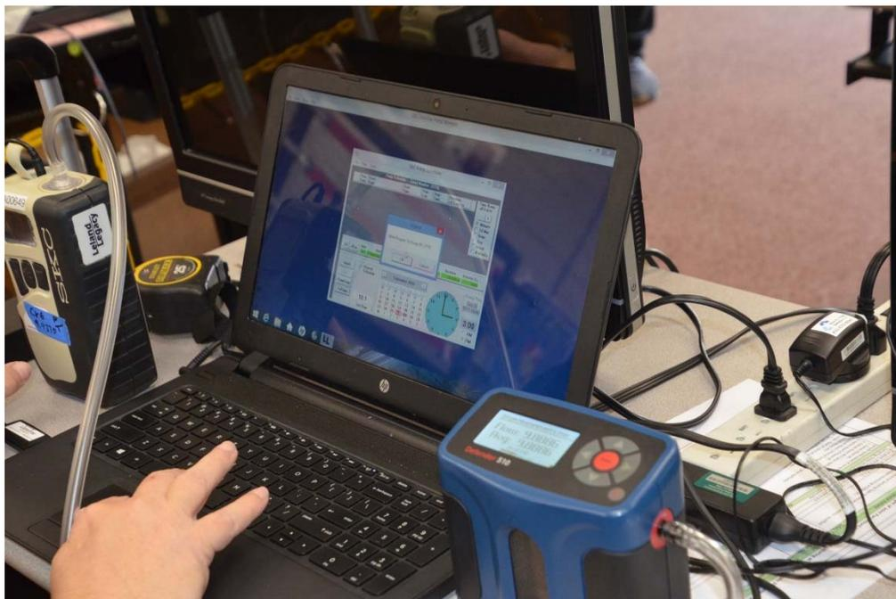
Photo 2 – Computer and pump set-up and interface with primary standard.
